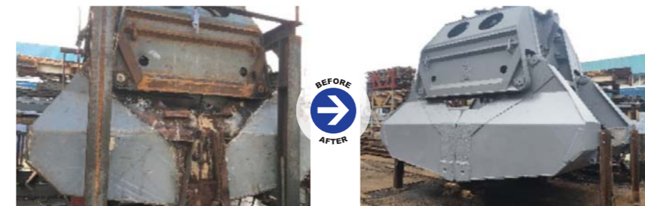
Damage repair of TOBU grab in workshop & anchorage.
