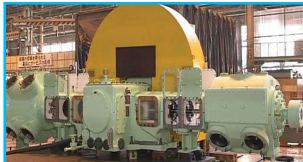
IHI Boil Off Gas Compressor
