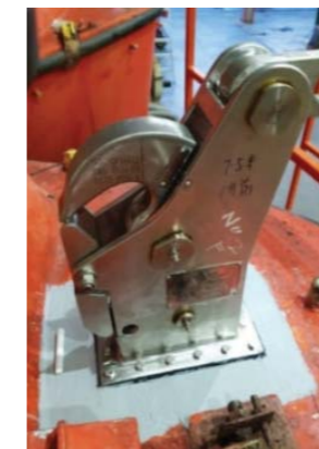
Lifeboat rehooking replacement with Fibre repair in workshop.
